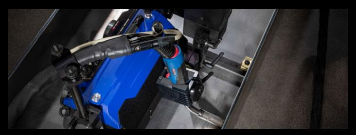
Clamping your own manual torch onto the welding tractor when welding long distances can be so easy: with the ABICAR POWER PAK. This system solution combines welding tractor, manual welding torch, TCP clamp and power source including wire feed unit. TCP – Tool Center Point – is a term used in automation and means working point.
